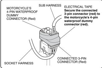
15. Stow the connected harnesses in the position shown.
