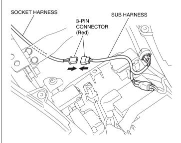
14. Secure the connected connector with electrical tape as shown.
