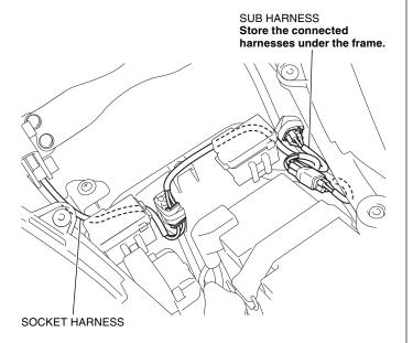
16. Bundle the socket harness with the wire tie as shown.
