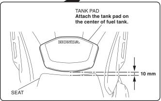
4. Apply adequate pressure to the attached tank pad.
