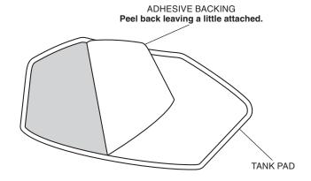
3. Attach the tank pad to the position shown.
