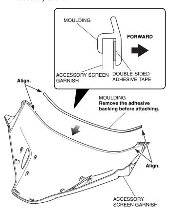
Clean the surface of the area shown using an isopropyl alcohol.
