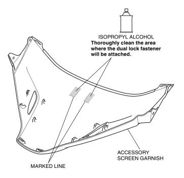
10. Install the dual lock fastener to the accessory screen garnish as shown.
