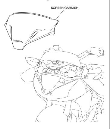
5. Remove the twist clips from the screen garnish as shown.
