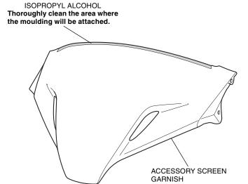
8. Install the moulding to the screen garnish of the accessory as shown.
