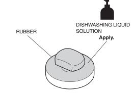
2. Install the rubber in the position shown.
