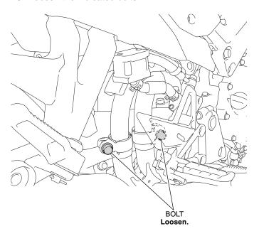
$26. \ \ \text{Remove the bolts as shown}.$
