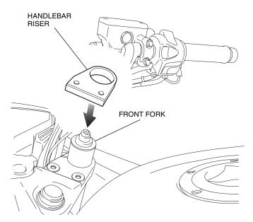
4. Install the right handlebar assembly in the reverse order of removal.
