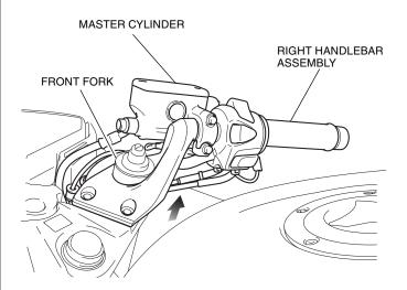
3. Install the handlebar riser as shown.
