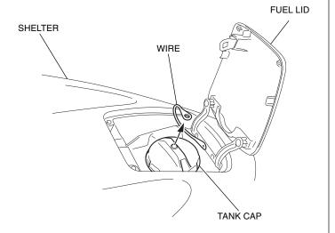
18. Disconnect the connectors and move the shelter to the rear of motorcycle.
