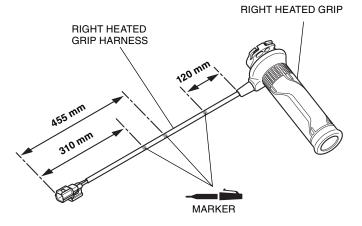
44. Wind the electrical tape on the marked position as shown.
