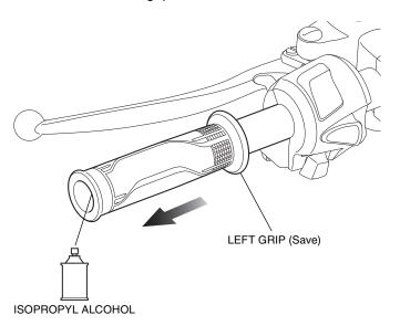
26. Using isopropyl alcohol, remove all traces of adhesive from the left handlebar.
