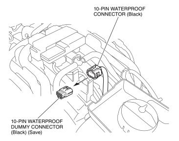
22. Connect the heater controller as shown.
