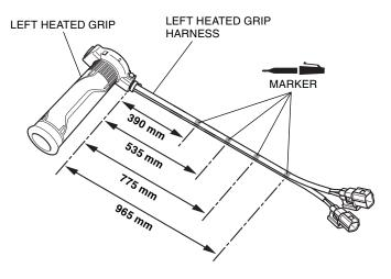
28. Install the clip bands and electrical tape at the marked positions as shown.
