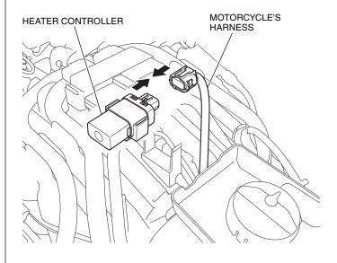
23. Secure the heater controller as shown.
