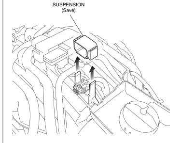
20. Install the suspension as shown.
