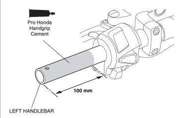
30. Spray isopropyl alcohol over the inside of the heated grip and outside of the left handlebar.
