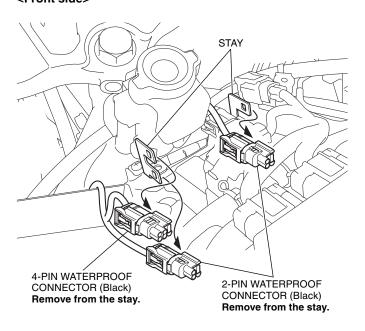
33. Remove the dummy connectors as shown.
