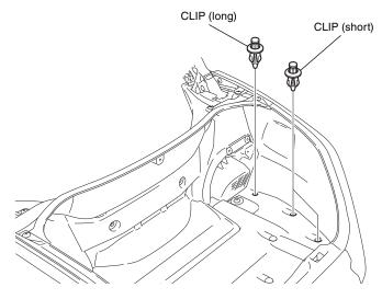
50. Install the trunk front lower panel as shown.
