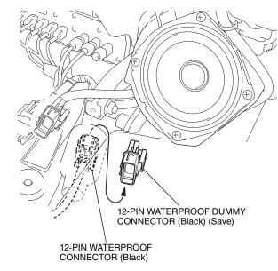
46. Connect the connector as shown.
