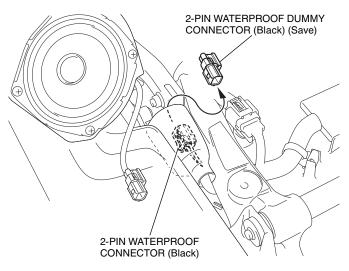
44. Connect the connector as shown.
