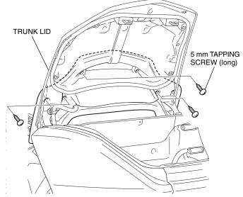
57. Install the 5 mm tapping screw as shown.
