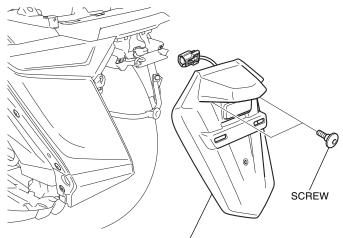
REAR FENDER Disconnect the connector.
