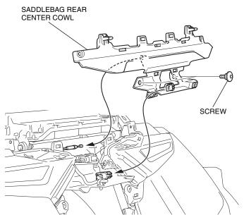
15. Remove the parts as shown.
