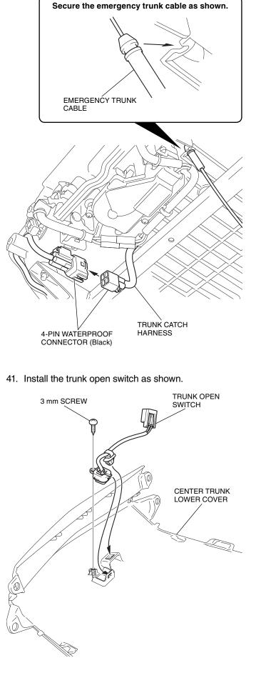
42. Connect the 2P black connector and install the trunk center lower cover as shown.
