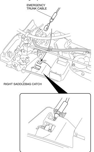
24. Install the radio antenna and right saddlebag catch in the reverse order of removal.
