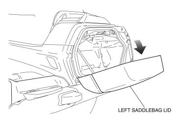
2. Remove the left side cover as shown, and disconnect the negative (-) cable of the battery.
