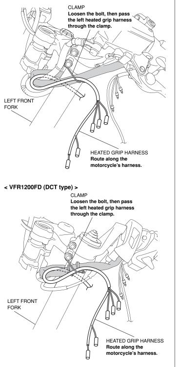
29. Fit the tube over the heated grip harness as shown.
