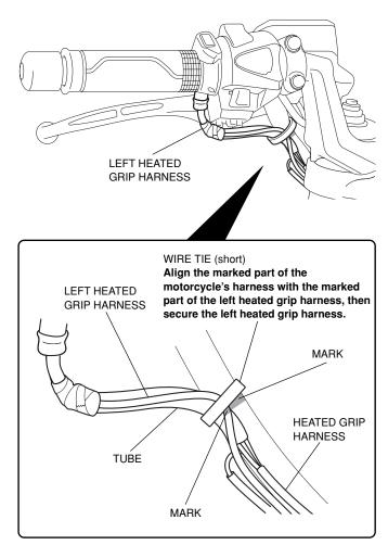
41. Secure the harness using a wire tie as shown.
