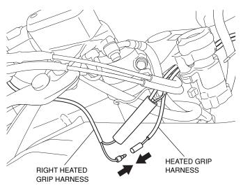
38. Wrap the shaded part with electric tape to secure the harness as shown.
