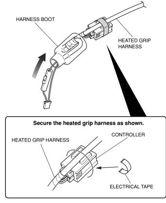
21 . Fit the boot over the controller as shown.
