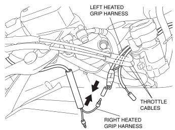
36. Move the tube over the plugged and taped connectors
