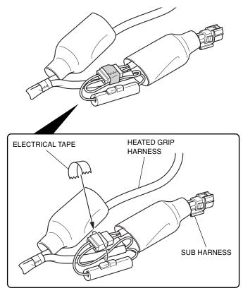
51. Cover the bound fuse and connector with the boot as shown.
