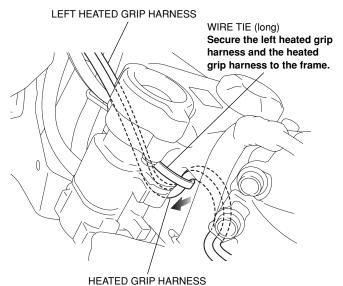
43. Secure the left heated grip harness and heated grip harness using the wire ties as shown.
