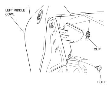
3. Remove the clips and bolt as shown.• Repeat on the right side.
