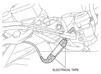
39. Measure and mark the left handlebar switch harness as shown.
