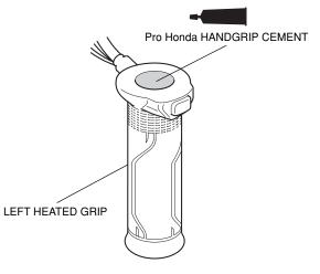
10. Apply Pro Honda handgrip cement to the left handlebar as shown.
