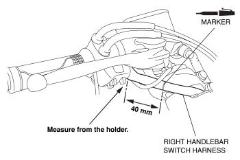
45. Secure the harness using a wire tie as shown.
