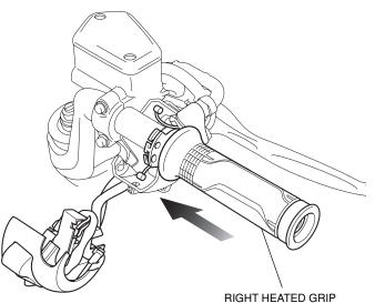
18. Reinstall the right handlebar weight as shown.
