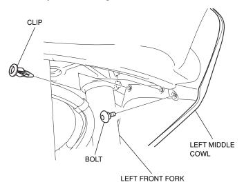
4. Using the procedures in the Service Manual for the motorcycle, remove the tank covers and middle cowls.
