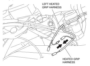
33. Wrap the shaded part with electric tape to secure the harness as shown.
