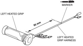
9. Liberally apply the Honda handgrip cement to the inside of the left heated grip from the kit as shown.
