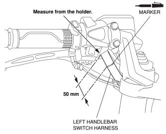
40. Secure the left heated grip harness in the position shown using a wire tie.
