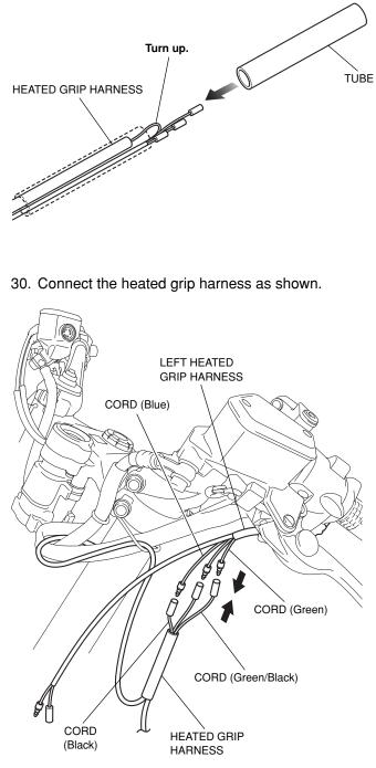
31. Secure the tube as shown.
