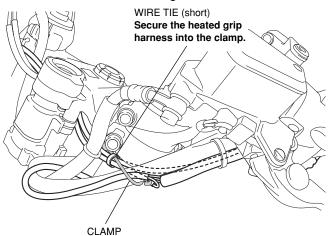
42. Secure the left heated grip harness and heated grip harness using the wire ties as shown.
