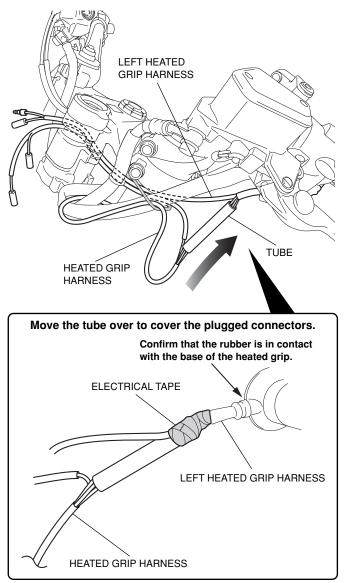
32. Route the left heated grip harness and the heated grip harness to the right side, then connect the heated grip harness as shown.
