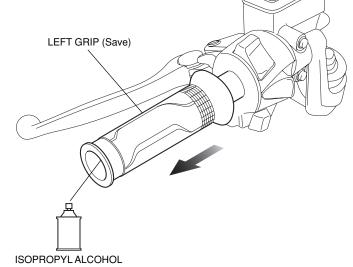
7. Using a isopropyl alcohol, remove all traces of adhesive from the left handlebar.
