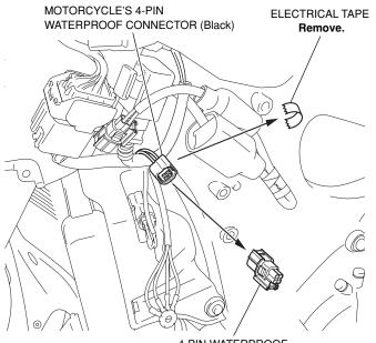
4-PIN WATERPROOF DUMMY CONNECTOR (Save) 54. Connect the sub harness to the motorcycle's harness as shown.
