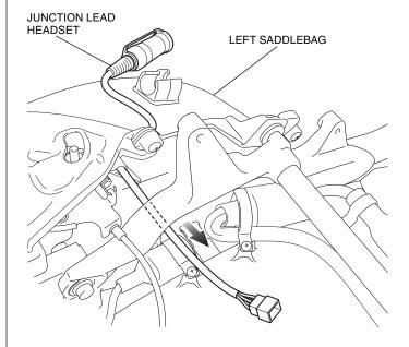
13. Connect the junction lead headset as shown.
