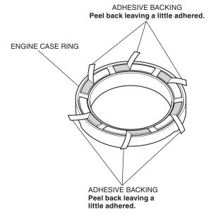
3. Attach the engine case ring as shown.
