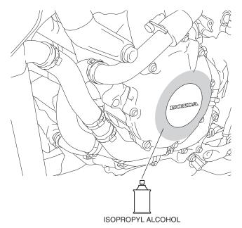
2. Peel off the adhesive backing on the engine case ring as shown.
