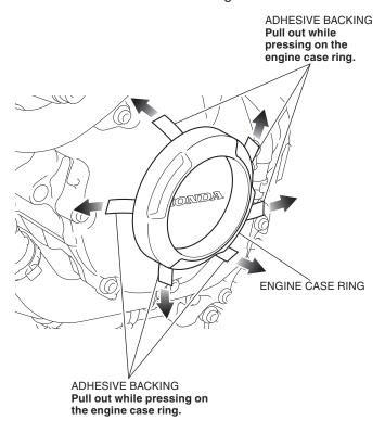
5. Apply adequate pressure to engine case ring.
