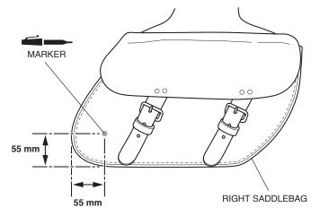
6. Using an electric drill motor and drill bit, drill a 8.5 mm hole through each of the marks you just made.
