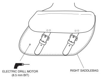
7. Install the reflector on the right saddlebag as shown.
