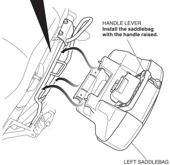
3. Lower the handle lever and lock the left saddlebag by turning the key counterclockwise as shown.
