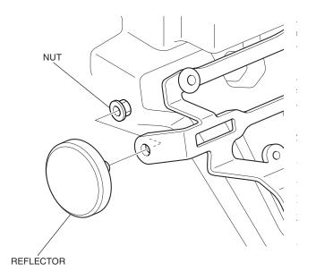
3. Install the reflector stay as shown.
