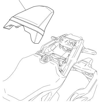
2. Pull the passenger seat straps out as shown.
