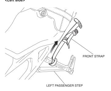
5. Route the front strap, and then secure the strap end as shown.
