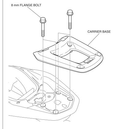
Install the carrier base as shown.
