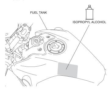
3. Attach the protection film to the fuel tank as shown.
