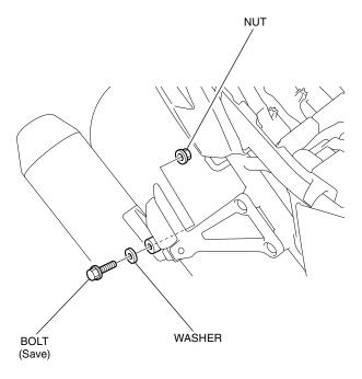
10. Loosely install the cross pipe as shown.
