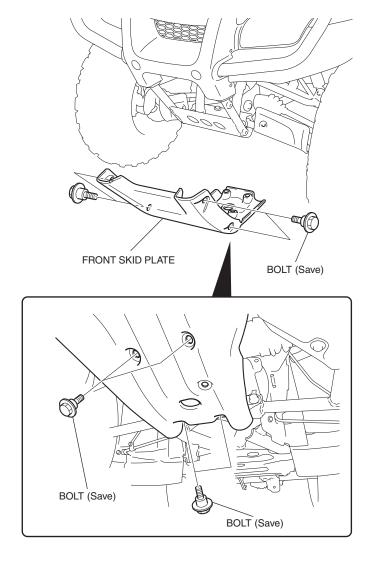
4. Install the front frame skid plate as shown.
