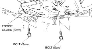
2. Remove the engine guard as shown.
