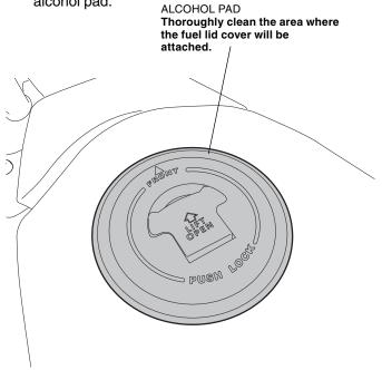
2. Attach the fuel lid cover by carefully aligning its inner and outer edges with the fuel lid.
