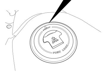
3. Attach the fuel lid ring and cap cover, making sure their contours are parallel with the edges of the corresponding motorcycle parts.
