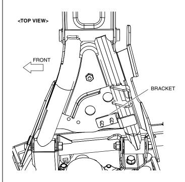
Install a 6 mm U-nut onto each screw as shown.
