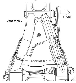
3. Place the guard onto the A-arm as shown.
