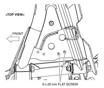
5. Install a bracket over the two inserted screws as shown.
