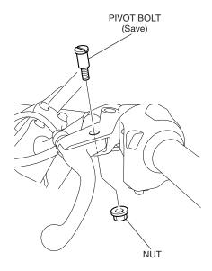
3. Install the left lever pivot bolt as shown.
