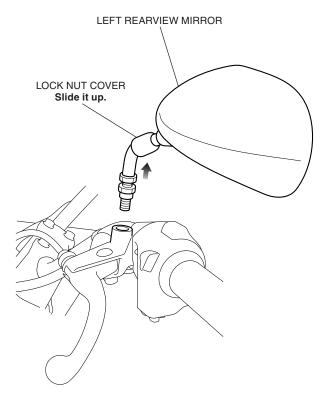
2. Remove the pivot bolt and nut.
