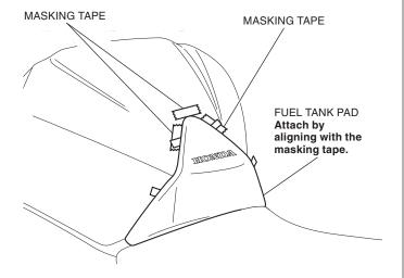
5. Remove the adhesive backing as shown.
