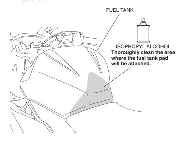
2. Arrange the fuel tank pad as shown and mark with masking tape.
