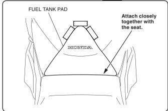
3. Peel off the adhesive backings on the fuel tank pad as shown.
