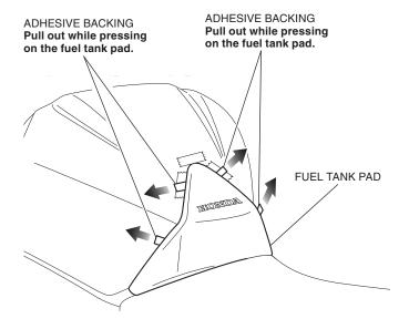
6. Remove the masking tape and apply adequate pressure to the attached fuel tank pad.
