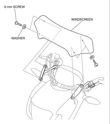
Align the windscreen assembly in accordance with the dimensions shown and check that the windscreen is positioned equally on both sides, then tighten the screws, bolts, and nuts to the specifications in the Torque Chart.
