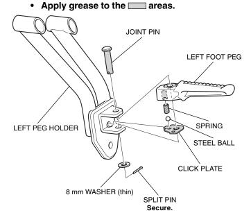
8. Install the left passenger peg holder assembly as shown.
