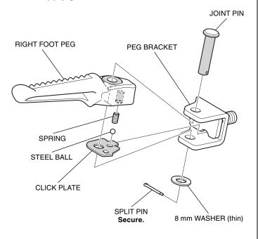
6. Install the right passenger peg assembly as shown.
