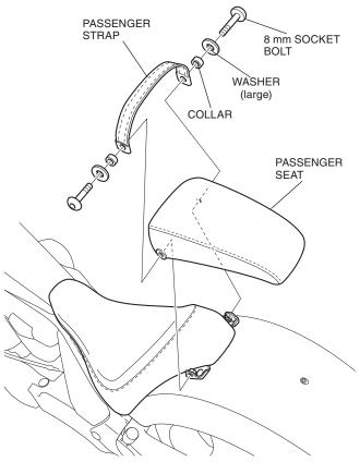
15. Install the parts as shown.
