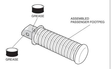
7. Install the left passenger peg bracket as shown.
