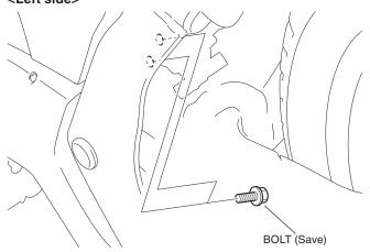
9. Install the assembled left passenger footpeg as shown.
