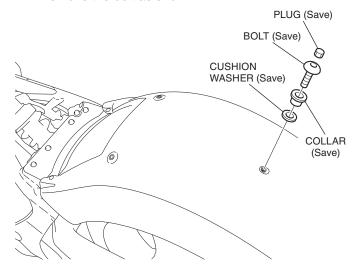
3. Remove the rear fender as shown.
