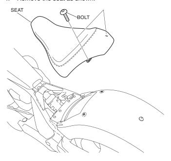
2. Remove the bolt as shown.
