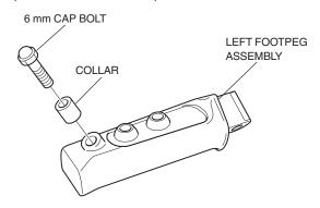
3. Remove the original equipment left footpeg assembly as shown.
