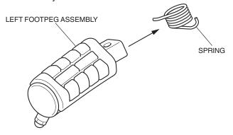
5. Install the spring to the new left footpeg assembly as shown.
