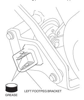
7. Install the new left footpeg assembly as shown.
