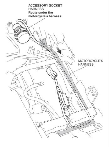
10. Install the connector clip as shown.
