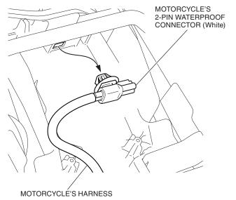
7. Remove the dummy connector as shown.
