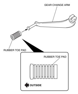
17. Install the gear change arm as shown.
