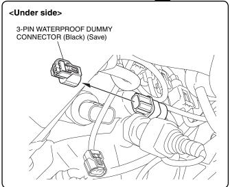
22. Connect the gear change unit harness as shown.
