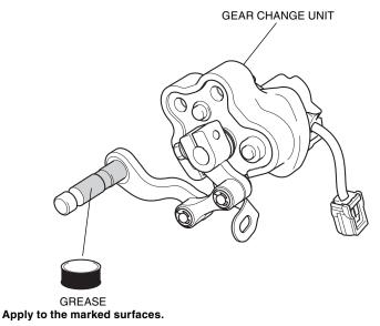
15. Loosely install the gear change unit as shown.
