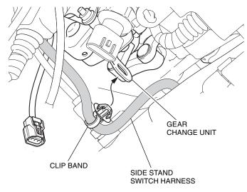
21. Remove the dummy connector as shown.
