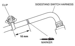
9. Remove the clip, and install the clip band as shown.
