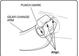
18. Install the 6 mm flange bolt as shown.
