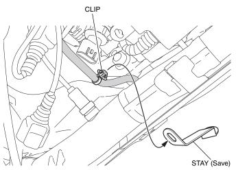
8. Mark the sidestand switch harness in the position shown.
