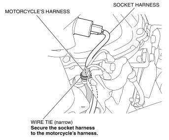
21. Secure the ACC harness with the wire tie as shown.
