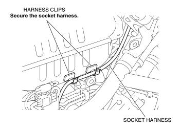
20. Secure the socket harness with the wire tie as shown.
