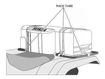
Secure each hook and loop strap around the rack tube.
