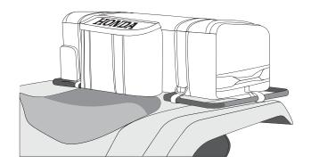
2. Identify the tubes that the bag will anchor to on the rear rack. Ensure that all hook and loop straps will reach a secure position on the rack.
