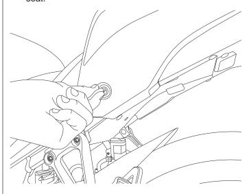
Remove the two 6 mm bolts securing the rider's seat. Remove the seat and save the bolts.
