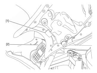
4. Secure the seat by installing a 6 mm washer [1] and the removed bolt [2] from Step 1. Repeat on the other side. Tighten the bolts to the specified torque in the Torque Chart.
