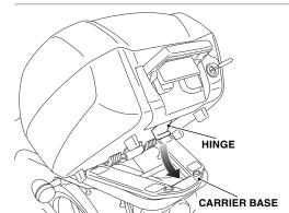
2. Position the hinge of the lock assembly on the carrier base as shown.
