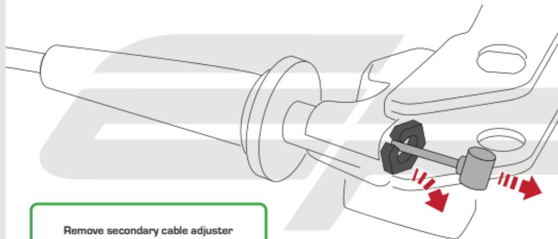
Remove secondary cable adjuster
