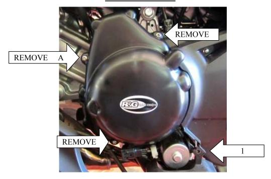
In this kit there should be: 1 x Engine Case Cover (ECC0133) 2 x M6x40mm long button head bolts 1 x M6x45mm long button head bolts
