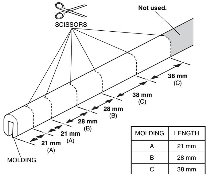
3. Attach the moldings to the cut part on the seat cowl as shown.
