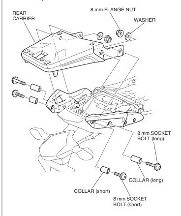
5. Tighten all loosely installed hardware to the specifications in the torque chart. Install the plugs as shown.
