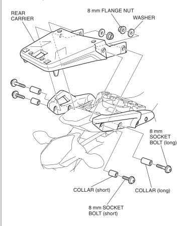
Tighten all loosely installed hardware to the specifications in the torque chart. Install the plugs as shown.
