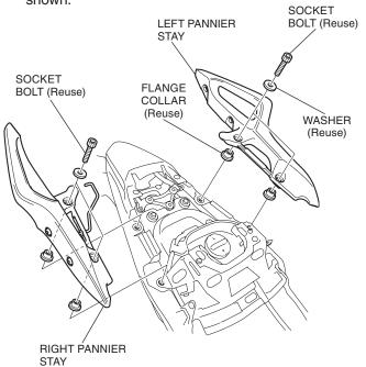
6. Loosely install the rear carrier as shown.
