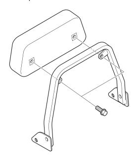
3. Loosely install the assembled backrest as shown.
