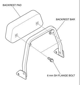
3. Loosely install the assembled backrest as shown.
