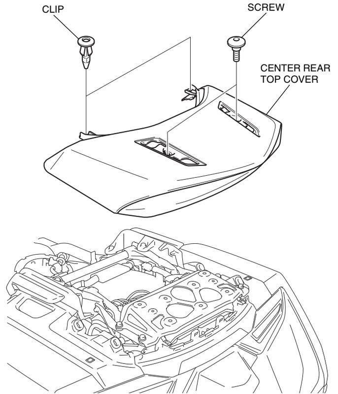
7. Remove the inner rear top cover as shown.
