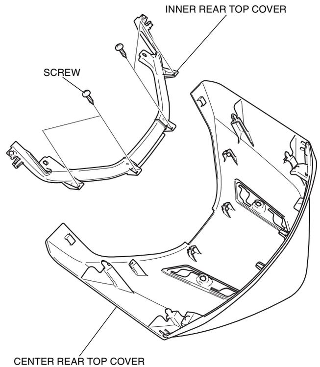
8. Drill at the marked lines of the inner rear top cover.
