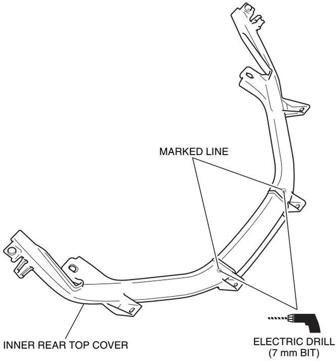
9. Cut out the
