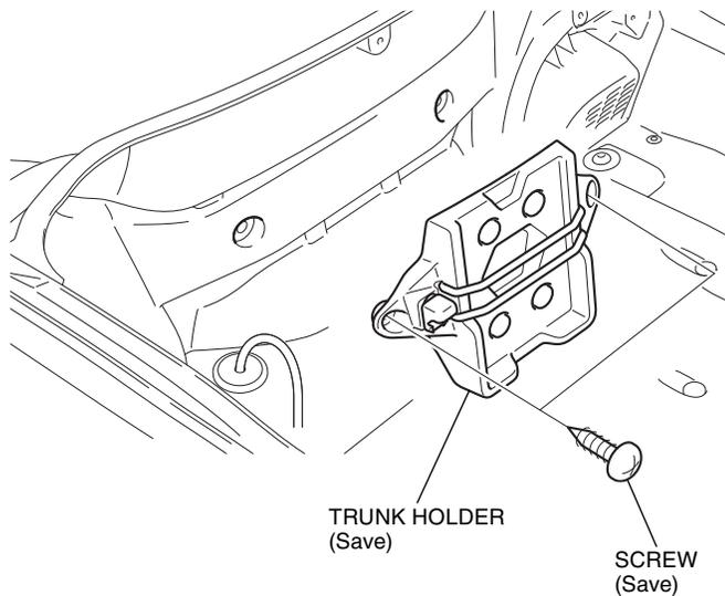
4. Install the 5mm screws as shown.
