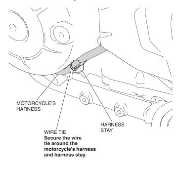
10. Mark the shift switch harness in the position shown.
