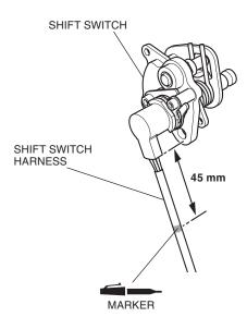
11. Loosely install the shift switch bracket to the shift switch as shown.
