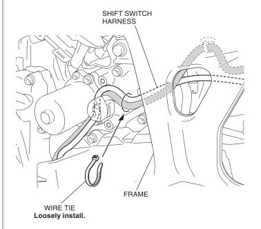
29. Secure the shift switch harness with the wire ties as shown.
