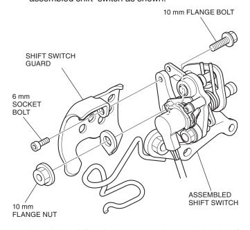
13. Install the shift switch cover on the assembled shift switch as shown.
