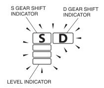
The S gear shift indicator, level indicator and D gear shift indicator blink alternately 5 seconds after deregistration is completed successfully. The shift switches can be released at this time.
