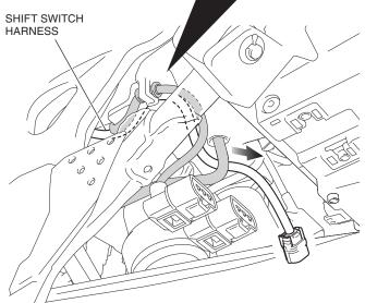
26. Connect the shift switch harness as shown.
