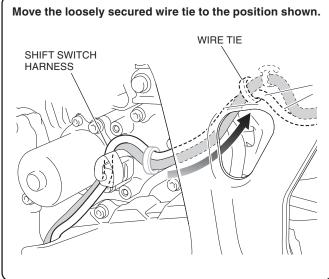
30. Secure the shift switch harness with the wire ties as shown.
