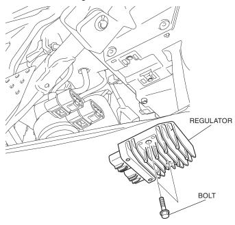
21. Remove the dummy connector as shown.
