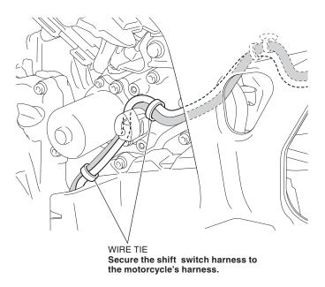
31. Secure the shift switch harness with the wire tie as shown.
