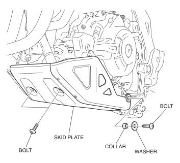
4. Remove the skid plate as shown.
