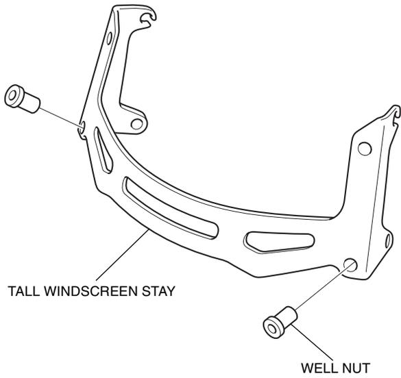
2. Install the grommets as shown.
