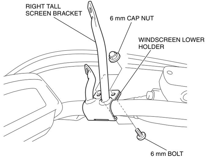
10. Reinstall the removed clamp.
