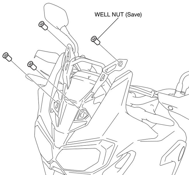
3. Install the well nuts as shown.
