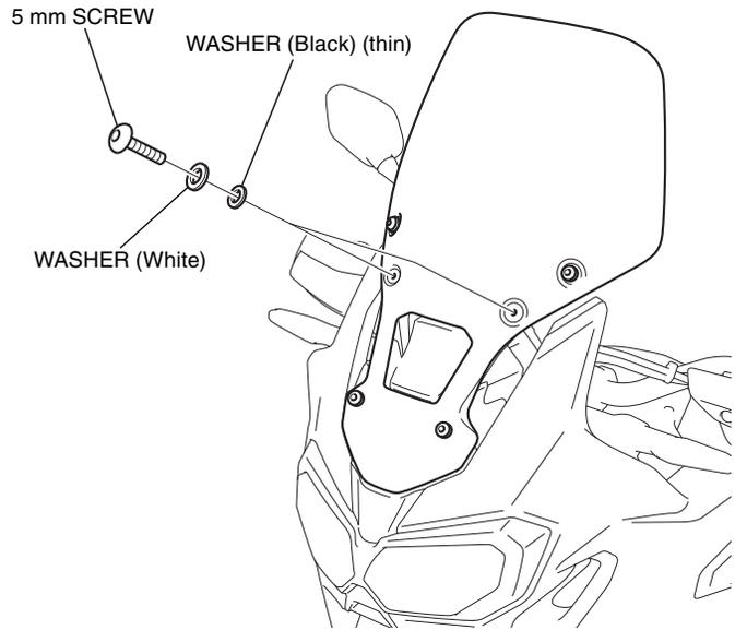
6. Tighten the loosely installed parts securely.
