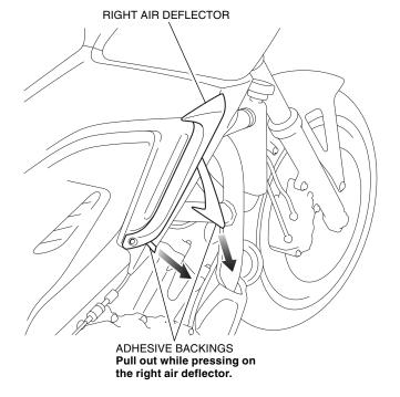
Apply adequate pressure to the attached right air deflector.
