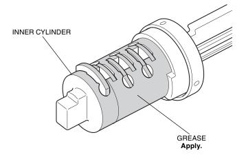
15 Install the inner joint into the cylinder body as shown.
