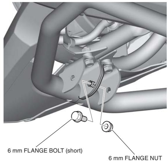
4. Tighten all loosely installed hardware.
