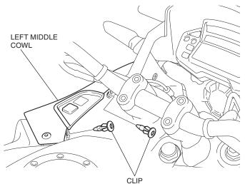
3. Remove the clips as shown. <Left side>
