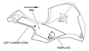
4. Remove the templates. Drill at the marked point shown using an electric drill.
