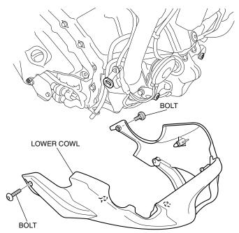
2. Refer to the Service Manual for the motorcycle, disassemble the lower cowls as shown.
