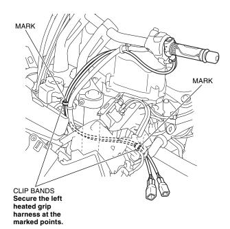
36. Connect and secure the left heated grip harness as shown.
