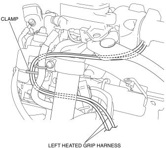
28. Secure the left heated grip harness using the wire tie as shown.
