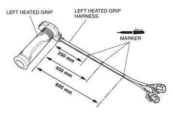
23. Install the clip band on the marked position as shown.
