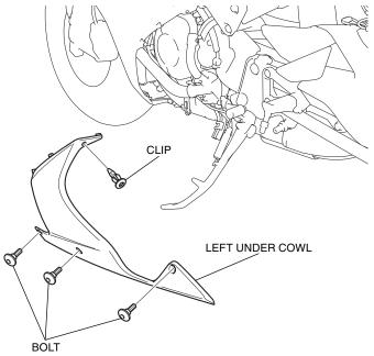
7. Remove the bolt and clip as shown.
