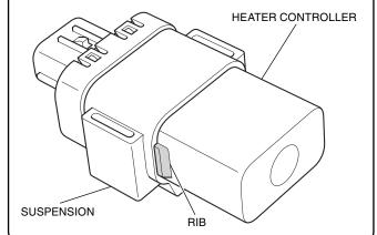
16. Remove the dummy connector as shown.
