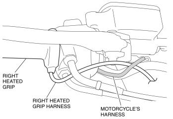
45. Secure the right heated grip harness using the wire tie as shown.
