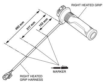
39. Wind electrical tape on the marked position as shown.
