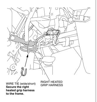
44. Secure the right heated grip harness with the wire tie as shown.
