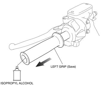
21. Using isopropyl alcohol, remove all traces of adhesive from the left handlebar.
