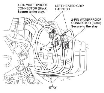
35. Secure the left heated grip harness using the wire tie as shown.
