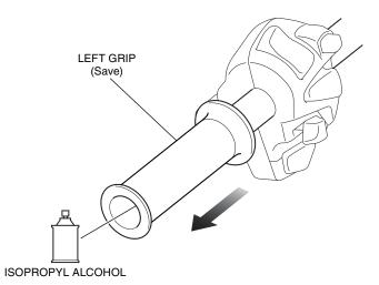
26. Using isopropyl alcohol, remove all traces of adhesive from the left handlebar.
