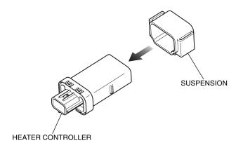
47. Connect and secure the heater controller as shown.
