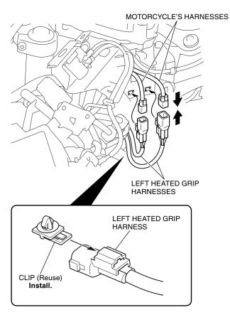
37. Bundle the left heated grip harnesses with the wire tie as shown.
