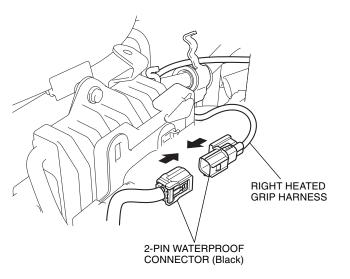
50. Secure the right heated grip harness using the wire tie as shown.
