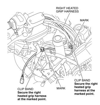
42. Connect and secure the right heated grip harness as shown.
