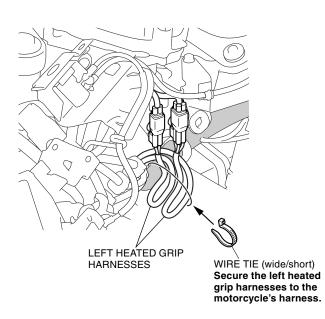
38. Remove the dummy connector as shown.
