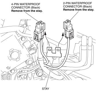
32. Remove the dummy connectors as shown.
