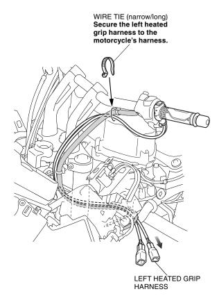
35. Secure the left heated grip harness to the clip bands as shown.
