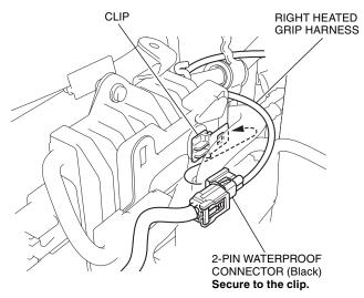
52. Secure the right heated grip harness using the wire ties as shown.
