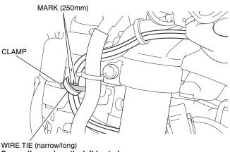
WIRE TIE (narrow/long) Secure the mark on the left heated grip harness to the clamp.
