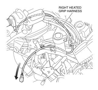
41. Secure the right heated grip harness to the clip bands as shown.
