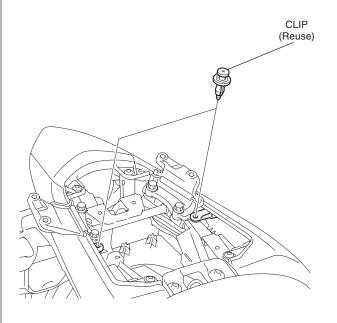
5. Install the rear carrier A as shown.
