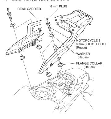
8. Install the motorcycle's parts in the reverser order of removal.
