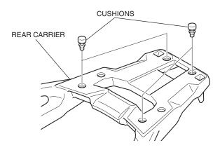
7. Install the rear carrier as shown.
