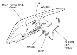
4. Install the pillion seat hinge to the right side of the rear carrier as shown.
